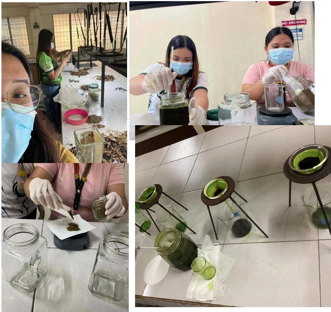
F.2. Preparation of Plant Samples Through Blending, Soaking, and Filtration
