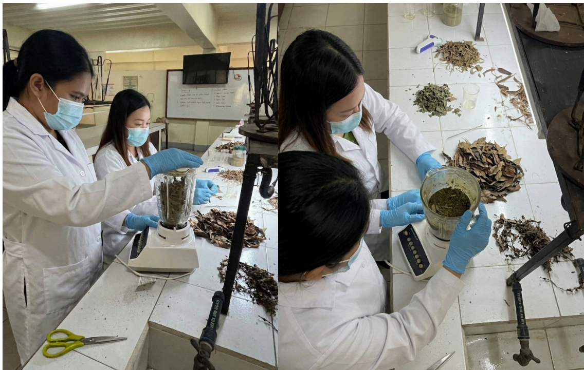
Figure 4. Pulverization of Dried Makataynuk Leaves Through Blending
