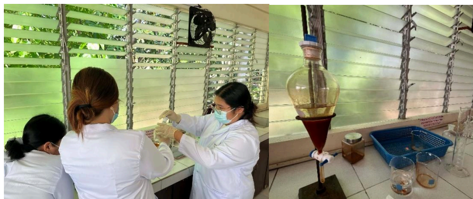
Figure 6. Solvent Partitioning and Extraction of Makataynuk Leaf Extracts.
