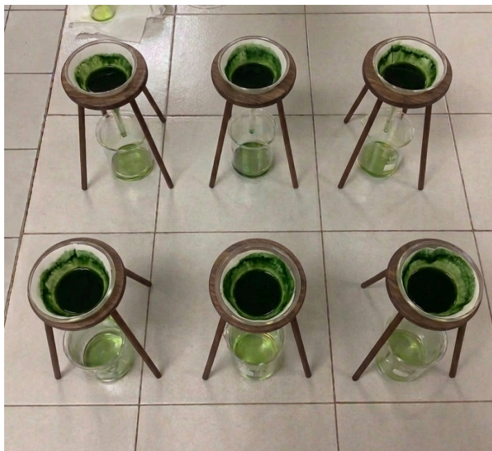
Figure 5. Filtration Process of the Soaked Makataynuk Leaf Extract
