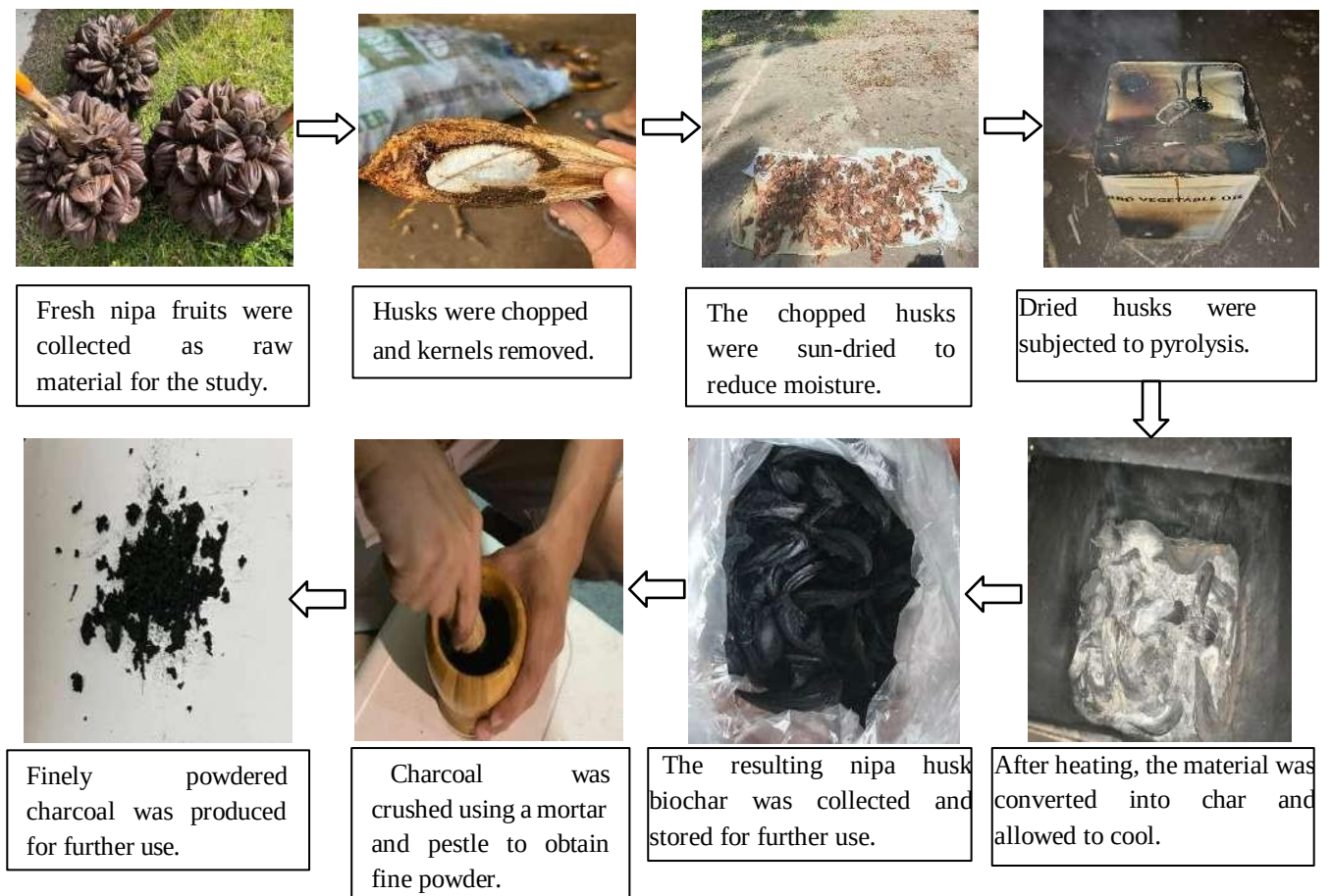
Figure 5. Procedure for obtaining charcoal from N. fruticans .
